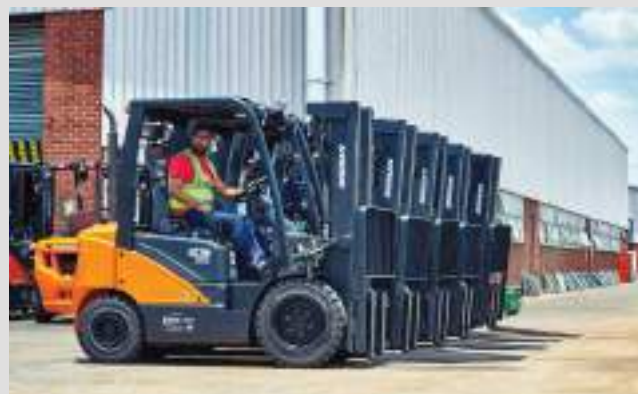
The Doosan forklifts from GLTC have capacities ranging from 1,8 to 7t.
